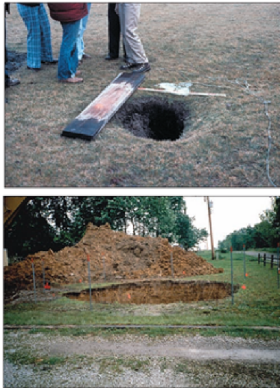
Figure 8 Diagram (Wildanger et al. 1980) and photographs of typical pit subsidence events.
