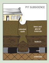
Pit subsidence forms a bell-shaped hole 6-8 feet deep and from 2-40 feet across and occurs when a shallow mine roof collapses.
